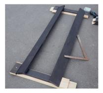
6. Screw the sides to the end cross pieces with the 50mm bugle head screws.
