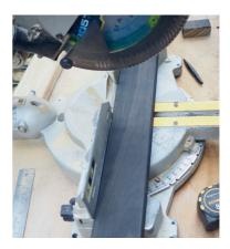
3. Cut the cross pieces to 550mm lengths then cut 30 degree chamfers, leaving a 5mm high face on the ends.
